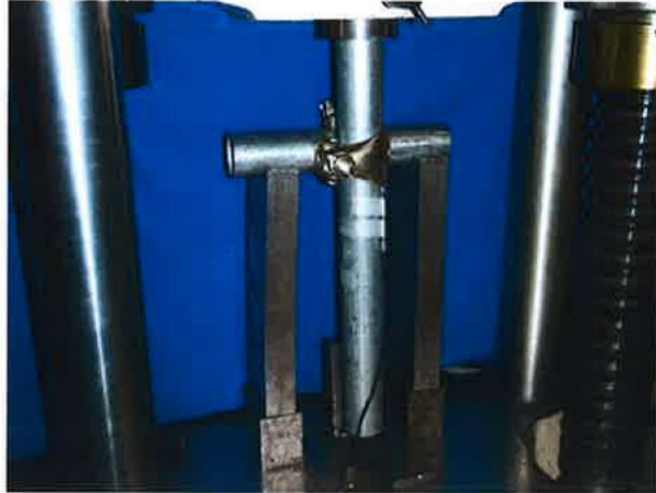
Photograph of Setup for Slipping Force
