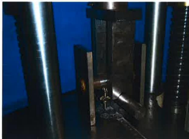
Photograph of setup for Pull Apart Force
